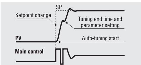
The **Natural frequency** method works best when the process variable is very near to the Setpoint. When activated, it causes a process oscillation around the Setpoint value.
