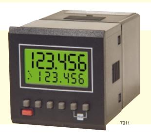
The LCD panel of this counter has two rows of 6 digits each. The upper characters are 7mm high and indicate the count value. The lower characters are 4mm high and indicate the preset point. It will count up to, or down from, the preset value and operate the output relay when the count reaches up to the preset or down to zero.
