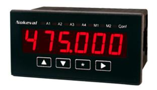
The panelmeter 2028 is specially designed to satisfy the needs of massflow indication in difficult applications where other flowmeters are unsuitable or difficult to use, such as measurement of solid matters or molten metal. Based on the current signal of a strain gauge transmitter the panelmeter 2028 calculates the change of the weight per second and in that way shows the actual flow rate.
