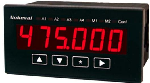
The panelmeter 2071 is designed for serial communication. It uses the simple Nokeval SCL protocol where only the address, value and check sum are sent. The panelmeter has both the serial inputs RS-232 and RS-485 as a standard. The serial bus is galvanically isolated from the processor and the power supply. In the configuration mode you can set the address, baud rate and the type of number value that you want to appear on the display after power connection.
