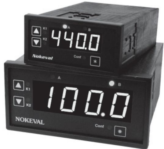
Indicators 440 and 441 have two separate input channels. You may set to both channels functions like square root, logarithm, subtraction, sum, etc. The channel, showing the calculation, may also have its own functions. You can freeze the automatic scanning or use only one channel. Many applications may be realized without separate transmitters e.g. differential temperature measurement or temperature compensation in flow metering.
