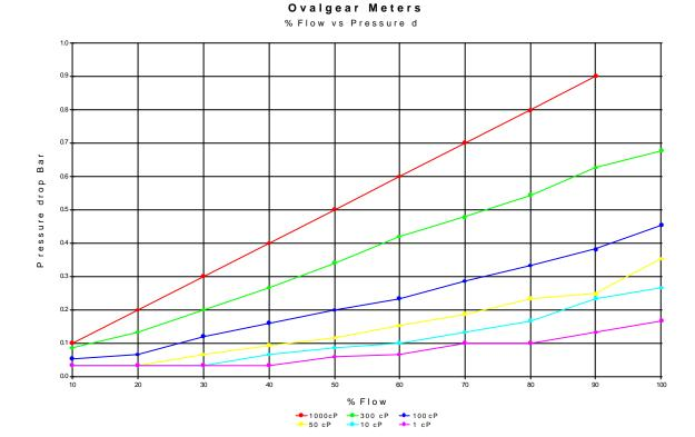
Higher viscosities may be accommodated but the flow range must be reduced e.g. for a viscosity of 2000 cP the maximum flow would be restricted to 80% of the full flow and for 10000 - 40% of full flow.
